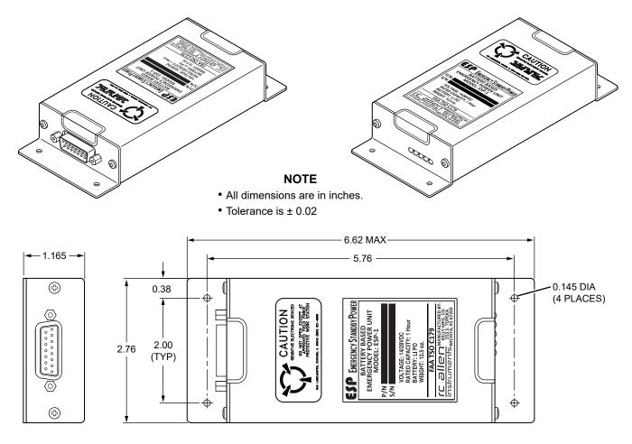
Figure 2.1, Battery Power Unit General Dimensions
